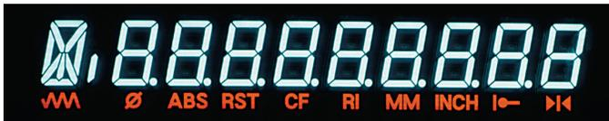
The Wizard readouts use VFD (Vacuum Fluorescent Display) technology for best readability. The axis designation is configurable. A set of indicators are provided for reference.
