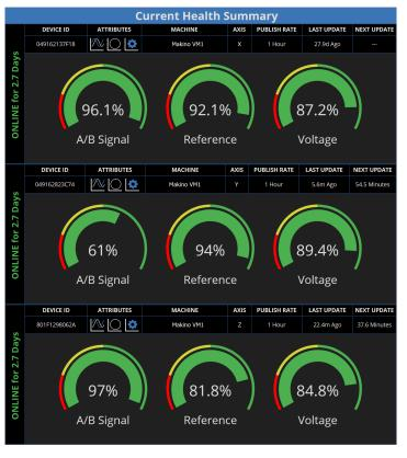
The Remote Detector series of devices are designed to be permanently installed in-line between the incremental scale and the control, allowing for real time analysis of scale conditions. Performance data and event information are transmitted using encrypted TCP/IP protocol over standard Ethernet to the MERIDIAN Cloud Service. Use of a Remote Detector is synonymous with having a trained technician watching your feedback system 24/7/365.
