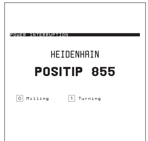
Fig. 37: POSITIP screen after initial switch-on
