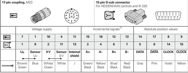
Cable shield connected to housing;  $U_P$  = power supply voltage
