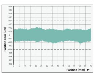
Position error within one signal period for a measuring range of 70 mm for LF encoders
