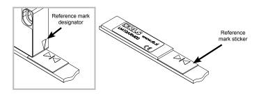
Remove the applicator tool leaving the reference mark sticker in the desired position.
