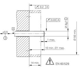
mm Tolerancing ISO 8015 ISO 2768 - m H < 6 mm: ±0.2 mm
