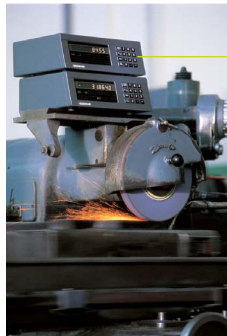
Grinding ND 221 B display unit Linear encoders on X and Y: LS 406 C Display step: 1 µm
