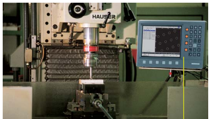
Drilling POSITIP display unit Linear encoders on X and Y: LS 406 C Display step: 1 \mu\text{m}
