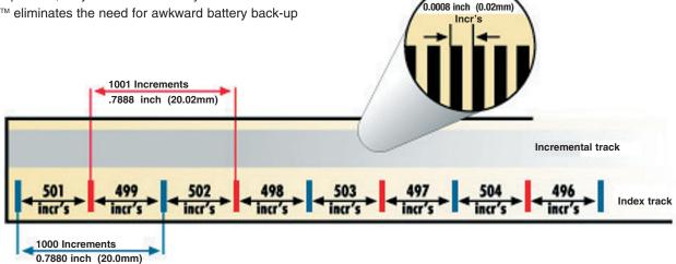
**THE EVERTRACK™** feature is accomplished by a reference index track in addition to the regular incremental grating, which is a set of lines .02mm apart. The index track has two sets of marks, indicated by blue and red. The distance between consecutive blue marks is always 1000 increments and between red marks, 1001 increments. So, along the index track there is always a unique number of increments between
