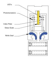
properties that provide the tight seal. Nitrile effectively resists absorption of shop chemicals making the seal very enduring.
