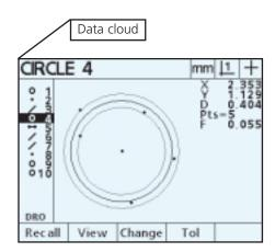
**Optical edge detection** Achieve higher throughput, more accurate measurements, and more consistent data with optical comparators using optical edge detection. Automatic point entry reduces operator subjectivity and fatigue.
