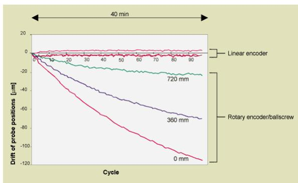
inch and you command your machine to move 0.5000 inches, then the machine will move until it reaches 5000 counts. Let's say that the scale has a dirty spot causing it to miss 50 counts. Well, the machine will still move until it reaches 5000 counts, but in this case, it will go 50 counts too far resulting in a position of 0.5050 inches.
