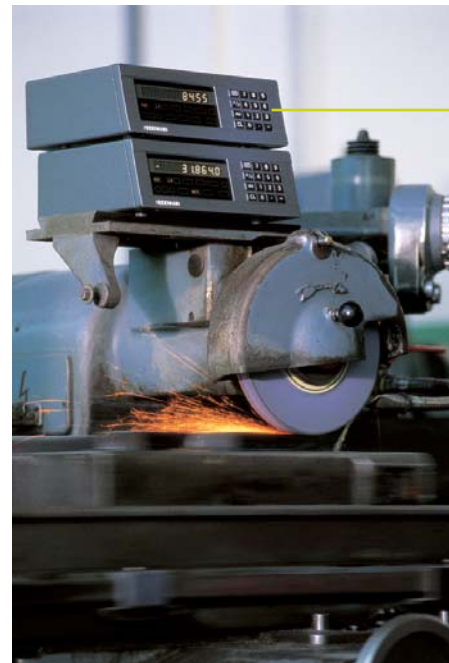
Grinding p. 14 ND 221 B display unit Linear encoders on X and Y: LS 406 C Display step: 1 µm
