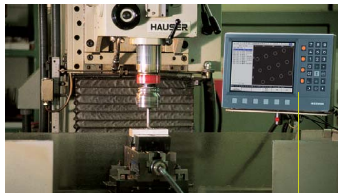
Drilling p. 10 POSITIP display unit Linear encoders on X and Y: LS 406 C Display step: 1 \mu\text{m}
