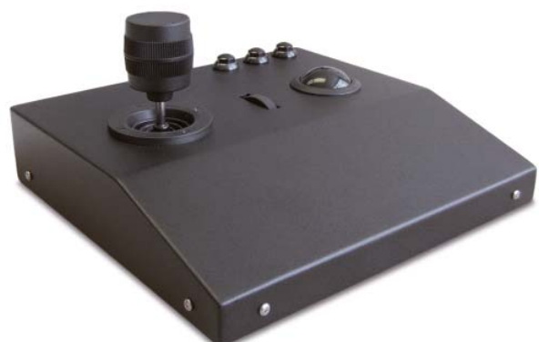
Joystick with trackball and Z-focus fine adjustment
