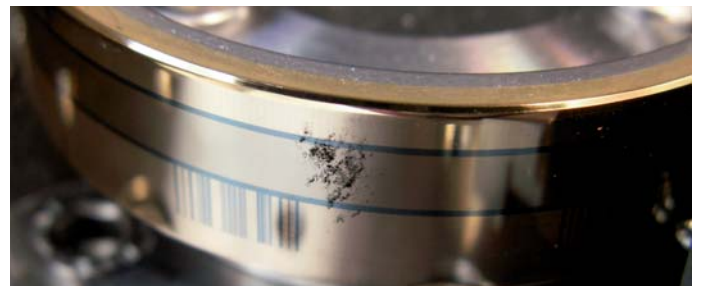
Contamination by fingerprint
