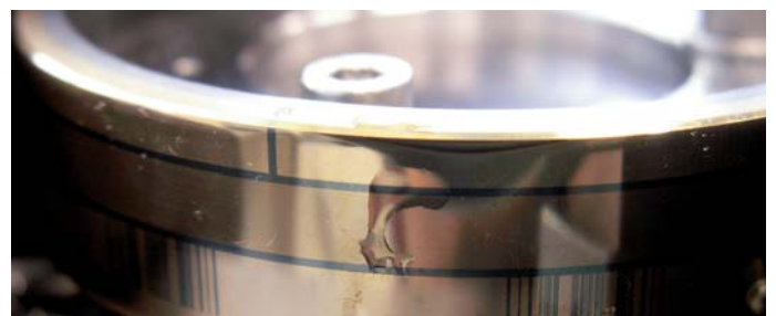
Contamination by toner dust
