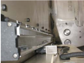
Heidenhain LS 187 precision linear scale integrated on the Viper VMC
