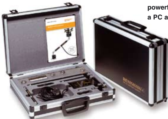
QC10 ballbar kit with Zerodur® calibrator
